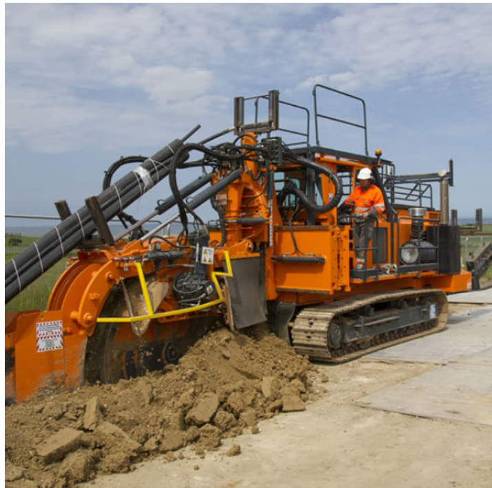
Plate 4-21: Example of cable trenching machine (Source: Equinor)
